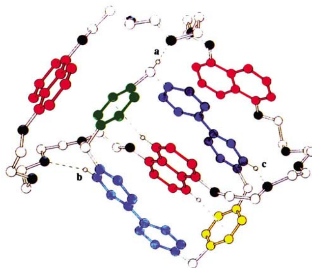
Fig. 1 The structure of 1 4+ in the solid state, showing the [C-H... \pi ] and [C-H...O] stabilising interactions. The [H...ring centroid] distances are both 2.53 Å and the [C-H...O] distances are 2.35, 2.44 and 2.34 Å for the a, b and c hydrogen atoms, respectively.
